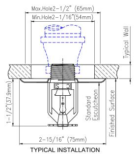
FIGURE C : MODEL NX025/NX026 PENDENT SPRINKLER INSTALLED WITH A STANDARD ESCUTCHEON
