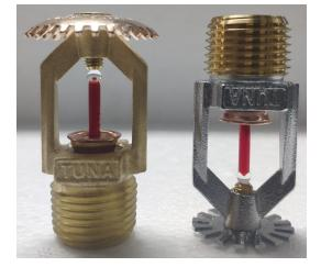
**D**uring a fire conditions, the thermal-sensitive liquid in the glass bulb expands, causing the bulb to shatter, releasing the button and spring seal assembly. Water flowing through the sprinkler orifice strikes the sprinkler deflector, forming a uniform spray pattern to extinguish or control the fire.
